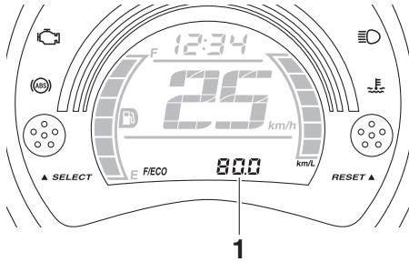
1. Instantaneous fuel consumption display
